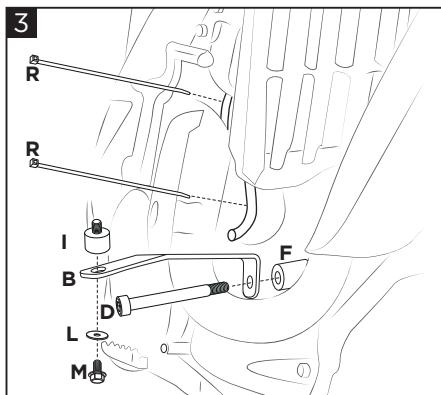
**Fit the right bracket (B) with the spacer (F) through the screw (D). Attach the other side of the bracket using the screw (M), the washer (L) and the anti-vibration device (I). Secure the tube using the clamps (R).**
