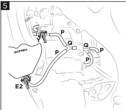
**Connect the tubes (P) to the cocks (E) and (Y) through the Y joints (Q).**
