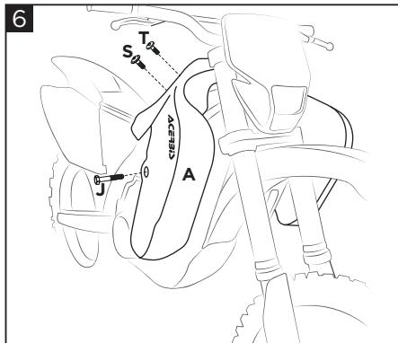
**Mount the Acerbis tank (A) on the motorcycle through the original screws (S) and (T). Use the screws (J) to reassemble the side panels.**
