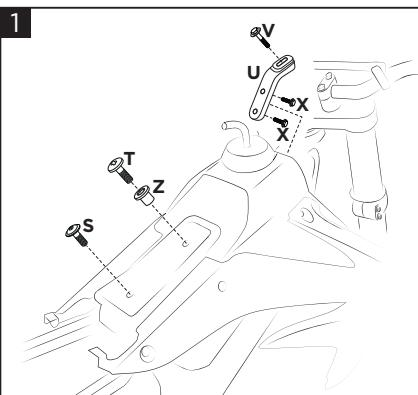
**Remove the original tank using the screws (T) and (S), the bushing (Z) and the bracket (U) with the screws (X) and (V).**
