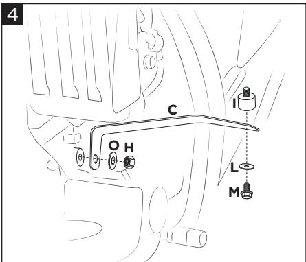
**Fit the left bracket (C) with the washer (O) and the nut (M). Attach the other side of the bracket using the screw (M), the washer (L) and the anti-vibration device (I).**
