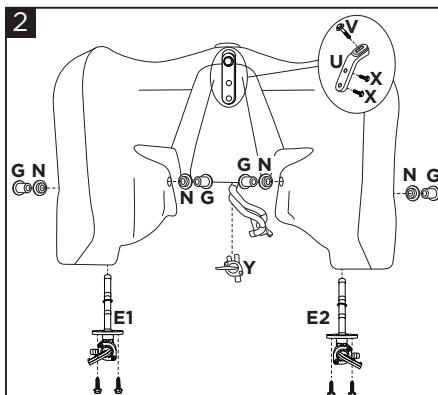
**Mount on the Acerbis tank (A) the bushings (G), the rubbers (N) and the cocks (E) and (Y).
